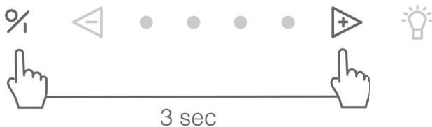
To switch the InTouch function off press the ① key and ② key at the same time for 3 seconds. The 2nd and 3rd LEDs flash 3 times to confirm. (The unit must be switched off).
