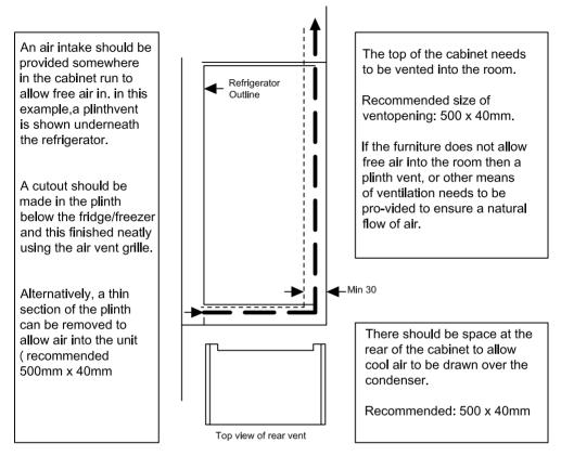
The open channel at the rear is clearly shown. For the correct operation of the appliance it is important that the top of the housing unit is not blocked off. A channel depth of 40-50mm is normal with most units.
