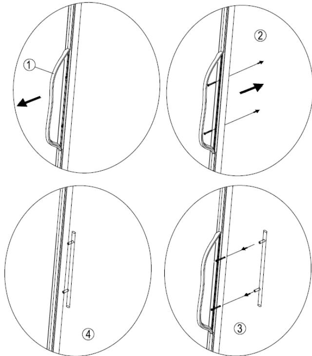
The device comes with one metal stainless steel handle. To install simply screw them to the door with the supplied screws.
